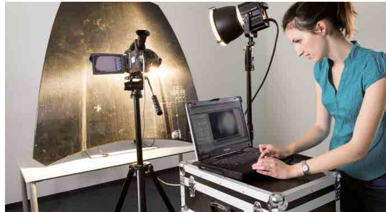
Did the front hood suffer from an incident? Non-destructive testing of the hood of a roadster would show material defects, since defects change the thermal flow in the material. This can be observed in the infrared spectrum
