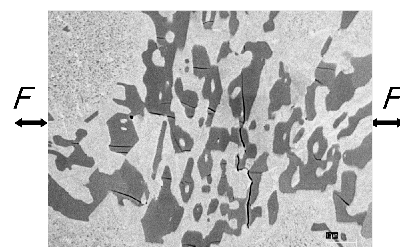
LCF specimen: long cracks perpendicular, short cracks parallel to the loading direction
