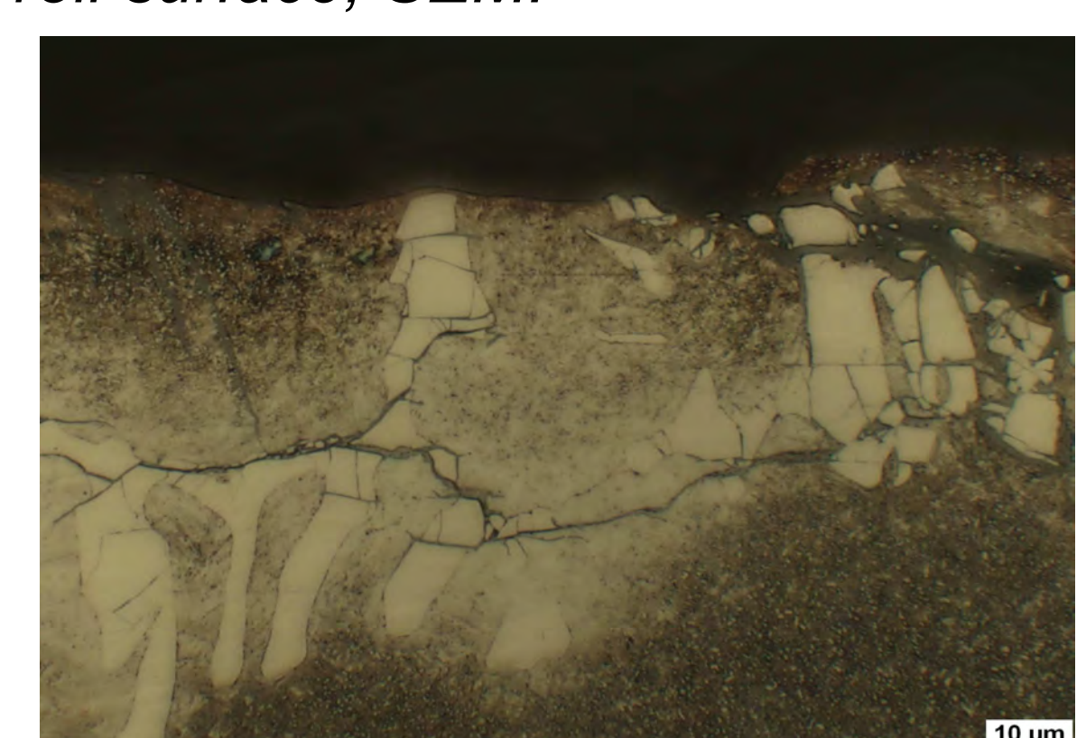
Carbides fractured parallel to the roll surface (light) and martensitic matrix (dark). LOM, Nital etching.
