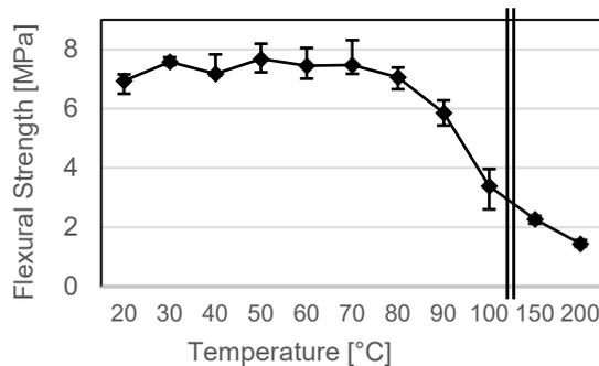
Fig. 2: Flexural Strength as a Function of External Temperature Load
