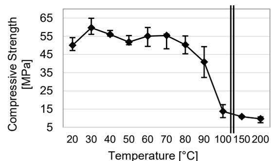
Fig. 1: Compressive Strength as a Function of External Temperature Load
